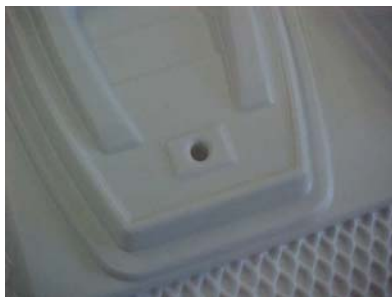
Figure 23. Improved locating hole for the adjuster.
