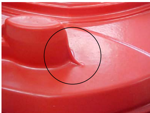
Figure 16. Failure - webbing due to the material of the forming overlapping
