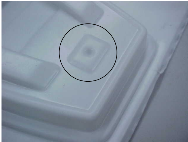
Figure 17. Failure – hole not deep or large enough to be formed for the sail adjuster
